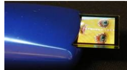
1.1" OLED displays of ca. 0.7 mm thin
