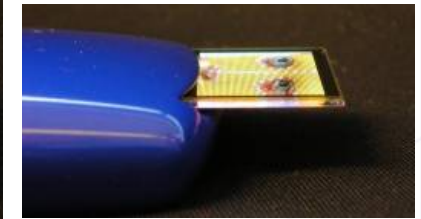
1.1" OLED displays of ca. 0.7 mm thin
